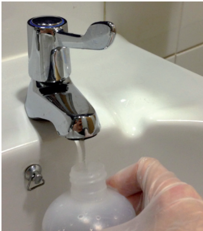
Figure 5.1: Aseptic Collection of Tap Water Sample
